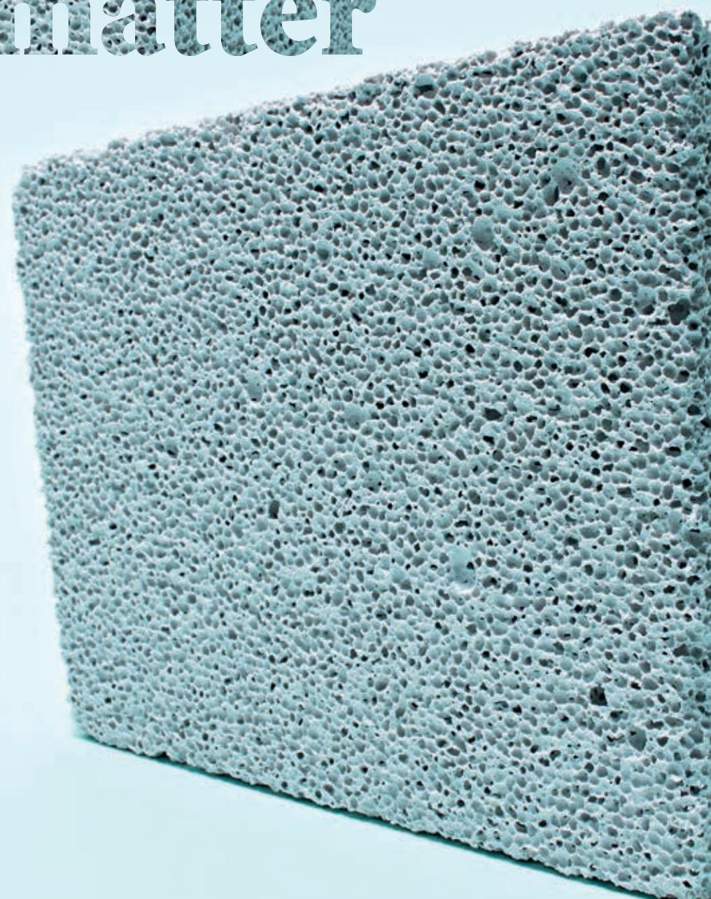
a temporary solution. It is thought that the collapses are usually triggered by weakening of the RAAC material following prolonged water ingress, often because of inadequate roof maintenance.
